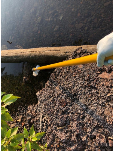
Pole grab sampler utilized to collect surface water samples.
