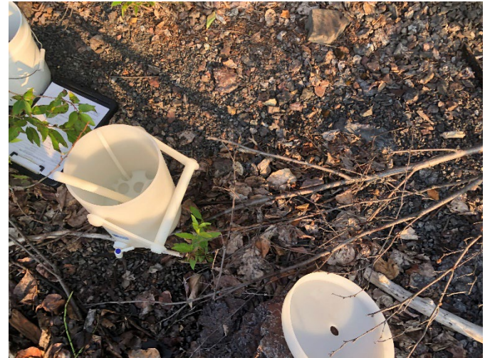
Churn splitter used for pouring sample water into for transfer to lab bottles
